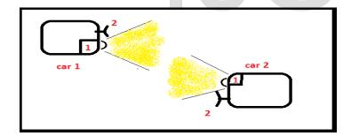
The above block diagram represents scenario of 2 cars approaching each other with Auto dim system fitted. The inputs to the system are photodiode and RF receiver (representing 1 and 2 in the above diagram). The output from the system is given to the headlights of the vehicles approaching and the lights are dimmed.
