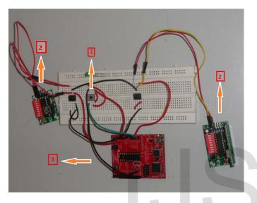
Opt 101 (1) – In this project OPT 101 is used for measuring the intensity of light and it act as one of the input to the system.
